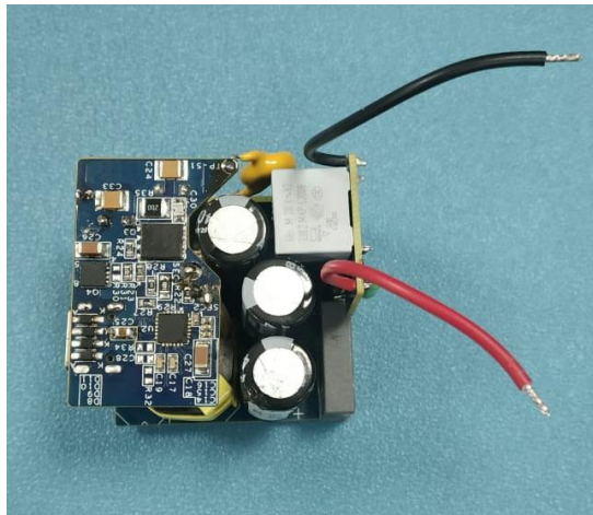
Figure 2.1-3 Top View showing Secondary side board
