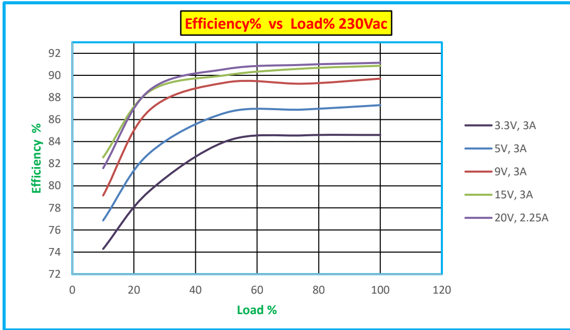
Figure 3.1-3 Efficiency at 230Vac, 50Hz
