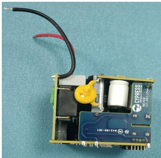
Figure 2.1-4 Side view showing EMI input filter board
